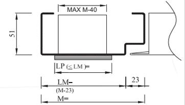
**RIVESTIMENTO**  completo  solo lato piano  solo lato vano (cabina) ACCIAIO INOX AISI-304 **SATINATO F7 (G220/240)** ACCIAIO INOX AISI-304 SCOTCH **BRITE** ACCIAIO INOX AISI-304 **RIGIDIZZATO**
